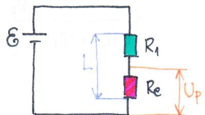
$$\frac{1}{R_e} = \frac{1}{R_2} + \frac{1}{R_p} = \frac{R_p + R_2}{R_2 R_p}$$
