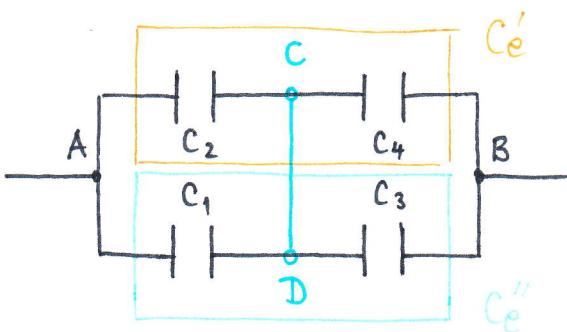
$$a) \frac{1}{Ce'} = \frac{1}{C_2} + \frac{1}{C_4} = \frac{C_2 + C_4}{C_2 C_4}$$
